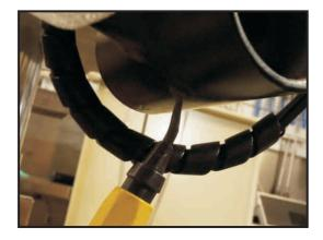
Be sure to deburr down the edges of the newly drilled hole, so that it doesn't nick the THUN wiring.
