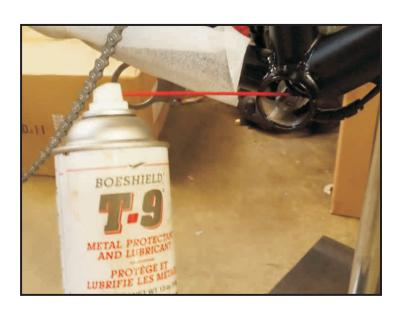
Next apply a good coat of Boeshield T-9 to the inside of the bottom bracket frame.
