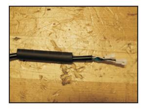
The final step is just to connect the included cable between the Cycle Analyst and the THUN sensor making sure to use the included heatshrink to seal the connection.
