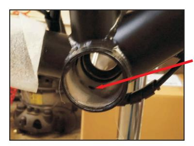
With the bottom bracket removed, you will be able to see a small hole in the bottom of the frame. This hole will need to be drilled out to allow the small white connectors on the THUN sensor to fit. A 7-8mm (5/16" - 3/32") should be sufficient.
