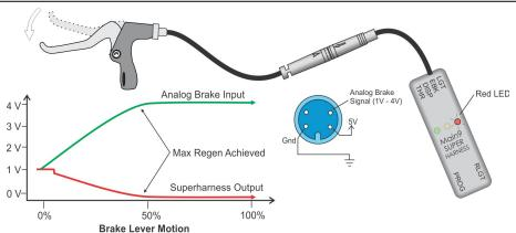
Figure 9: The analog brake lever has the same 1V - 4V nominal ouput as a throttle. The Superharness remaps this into a 0.8V - 0.0V regen command.
