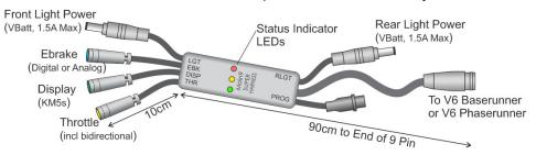
Figure 2: Superharness contains active circuitry
