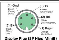
The display plug uses a 5 pin Higo connection\* wired in one of the more common of several known pinout standards.
