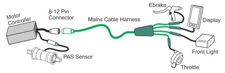
Figure 1: Example of a Mains Harness (Green)
