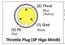
The throttle hookup is a conventional 3 pin Higo standard and expects to see a hall-effect throttle with a ~0.9 to 4.2V command signal range.
