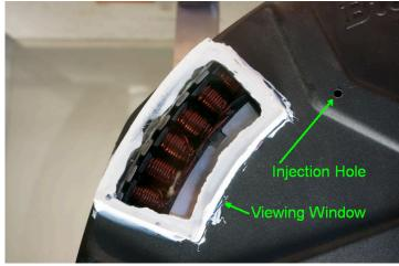
The motor was similarly tested 100, 200, and 300 rpm with Statorade added in 1mL increments while measuring the core to shell conductivity and drag torgues.
