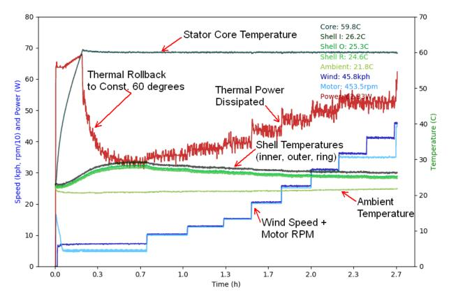
For the data analysis, we assumed that the motor can be characterized as two distinct thermal masses, the motor core and the motor shell. Heat is generated inside the motor core, and must first travel to the motor shell. As the shell warms up, it is then able to shed this heat to the passing ambient airflow.
