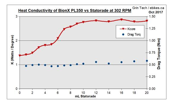
From this data, we can conclude that a total injection quantity of 8-10mL would be adequate to produce full thermal motor benefits over the typical wheel speed range of an ebike. This quantity would have no detectable increase in drag torque at normal cruising speeds, and only a very slight increase at low speeds with the motor spinning at 100 rpm and below.
