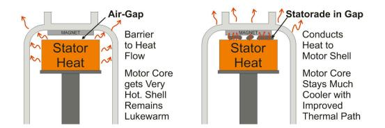
Since the initial release as a product, we have seen Statorade used to very good effect in a number of ebike applications where people have been reaching the thermal limits of a motor. This includes hub motors used in cargo bikes and
