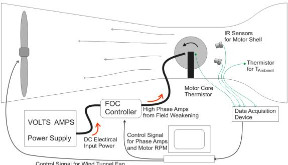
Control Signal for Wind Tunnel Fan
