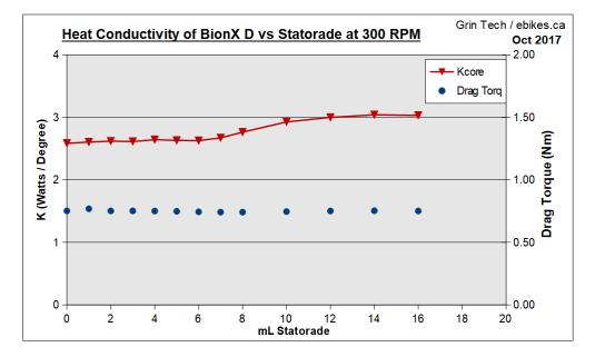
We can infer that at 300 rpm in such a large diameter motor, most of the Statorade was displaced by centripetal forces and was not bridging the gap between stator and rotor. That explains the lack of increased wheel drag and the reduced thermal effects.
