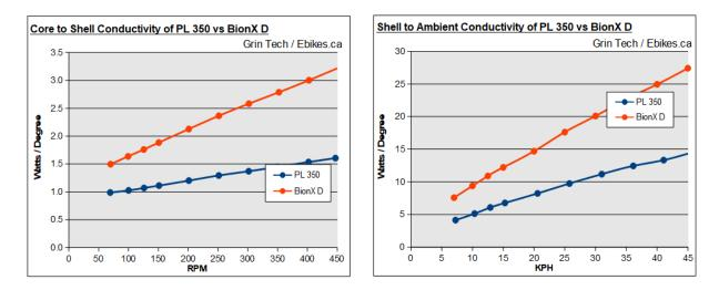
Notice that on both PL350 and D Series hubs, the Shell to Ambient conductivity is many times higher than the Core to Shell conductivity. That means the primary barrier to heat flow out of the motor is getting it from the motor stator to the shell. Once heat is on the motor shell, it transfers easily to the ambient air.
