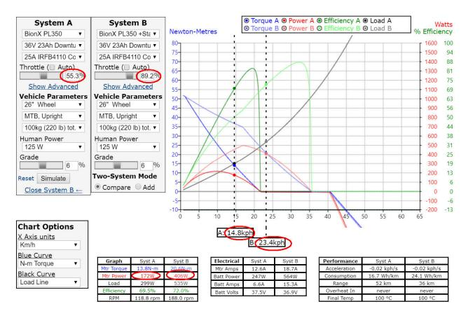
In this thermal rollback scenario, the rider with a stock PL350 would end up climbing the hill at 14.8 kph with the motor only contributing 172 watts of propulsion. Meanwhile, that rider pedaling with the same effort on the bike with Statorade would be climbing uphill much faster at 23.5 kph, with the motor contributing over 400 watts of power.
