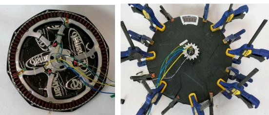
Nevertheless, we were able to reassemble and seal the modified motor and added a clear acrylic window to the motor side cover as a viewing port to see inside.
