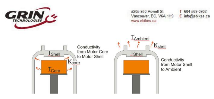
This provides two heat conductivity terms. The first  $K_{core}$ , from the motor core to the motor shell, we expect to vary with motor RPM, while the second,  $K_{shell}$ , we expect to vary mostly with the passing wind speed. In general the motor RPM and wind speed are related by the wheel diameter, though in the wind tunnel we could vary these independently.
