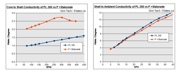
The thermal conductivity from the motor shell to the ambient air (right graph) is of course not affected much by the presence of Statorade. However the net conductivity from core to ambient shown below is still markedly improved, with an average 80% increase in heat transfer from low speeds up to 300 rpm. The Statorade enables the small PL350 motor to have almost exactly the same heat shedding abilities as the much larger 'D' series hub.
