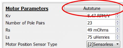
With the software connected, the next step is to run the Phaserunner “Autotune” routine. This will cause the motor to spin, and it is essential that your bike is propped up so that the motor can freely rotate both forwards and reverse. With a rear hub motor be sure that the cranks can turn completely and won’t collide with a kickstand for example, in case the initial testing spins the motor backwards.
