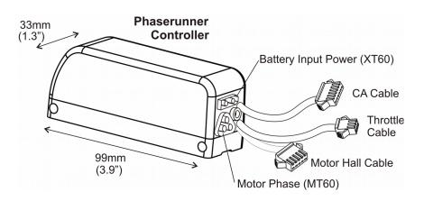
However, unlike standard trapezoidal or sinewave controllers, the Field Oriented Controller (FOC) needs to be tuned to the specific motor that it is paired with. For that you need the USB->TTL communication cable and a computer with the Phaserunner software suite installed. You cannot just connect the phase and hall wires to a random motor and expect it to run.
