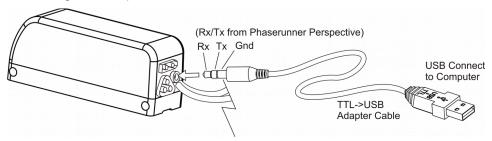
The communication standard uses a 5V TTL level serial bus, and Grin produces a 3m long TTL->USB adapter cable so that you can connect with the USB port of a standard computer. This is the same communication cable used with the Cycle Analyst and Satiator products. You can also use 3rd party USB->Serial cables, such as FTDI's part number TTL-232R-5V-AJ.
