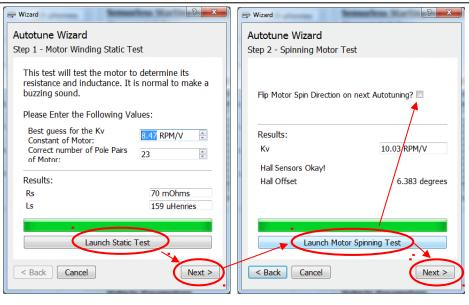
During this spinning test, the Phaserunner will be self starting the motor in sensorless mode. If the motor fails to spin and just starts and stutters a few times, then you will need to adjust the sensorless starting parameters as described in section 4.4 until the motor is able to self start OK.
