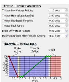
By default, the Phaserunner will be configured so that active throttle starts at 1.2V, and full throttle is reached at 3.5V, which is broadly compatible with Hall Effect ebike throttles. The Phaserunner has an analog ebrake line which is tied to the throttle line, and the regen voltage is mapped so that regenerative braking starts at 0.8V and then reaches maximum intensity at 0.0V.
