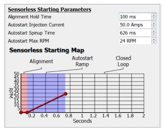
As a starting point, you should use an autostart injection current similar to your maximum phase current, an Autostart Max RPM about 5-10% of the running
