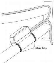
The Phaserunner is designed to be narrow in width and has a channel down the back of the heatsink so that it can be strapped to your bicycle tubing with a pair of cable ties. When mounted externally like this, the controller is exposed to abundant air flow for cooling and the on-off button remains accessible
