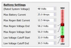
With the controller mapped to your motor and spinning fine, you should next set the battery voltage and current settings to appropriate values for your pack. We recommend making the max regen voltage the same as the full charge voltage of your battery, with the regen start voltage about 0.5V less. For the low voltage rollback, you can set this to be just above the BMS cutoff
