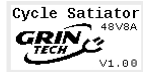
Figure 2: Splash Screen after power applied, shows Model and Firmware Version
